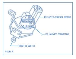
Do not jump the ISC motor after the plunger reaches the fully-extended or retracted position
